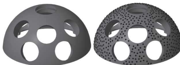
Figure 8: Three dimensional model before and after application of friction bumps
