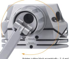
Rotates cutting block eccentrically - 2, 4 and 6mm
