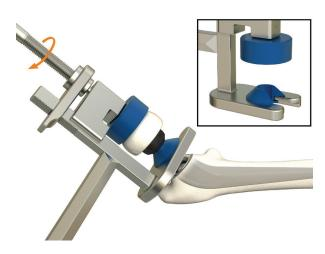
If the insert and the ball head have to be adjusted in situ (e.g. during revision of a monobloc stem) replace the plastic part underneath the head/liner inserter with the Neck Adaptor for Monobloc Stem (21000503/75017087). Then place the instrument on the neck of the monobloc stem, put the PE or XLPE insert onto the ball head and turn the T-handle until the head is completely locked into the PE or XLPE insert and moves freely.
