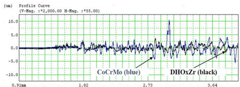
Figure 13: Representative surface profile traces within wear track on disks from 20 cycles of 300lb load. OXINIUM DH (DHOxZr) and CoCrMo show comparable damage resistance.<sup>35</sup>
