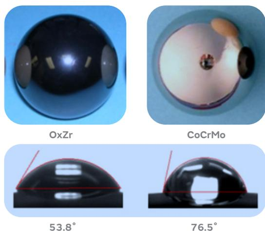
Figure 9: OxZr surface was more wettable than CoCrMo.
