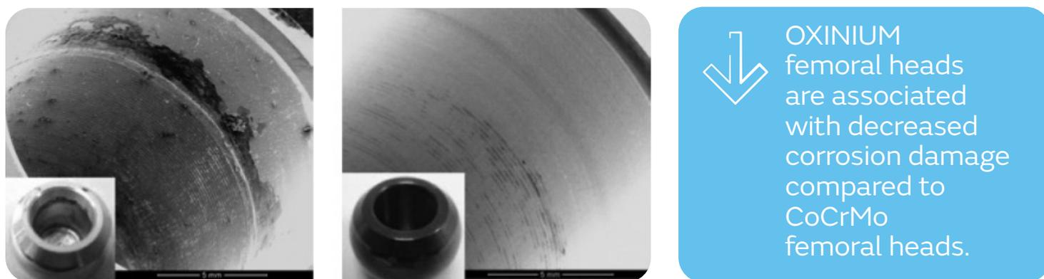
**Figure 7:** SEM image of worst case CoCrMo taper (at left) and worst case OXINIUM (at right).
