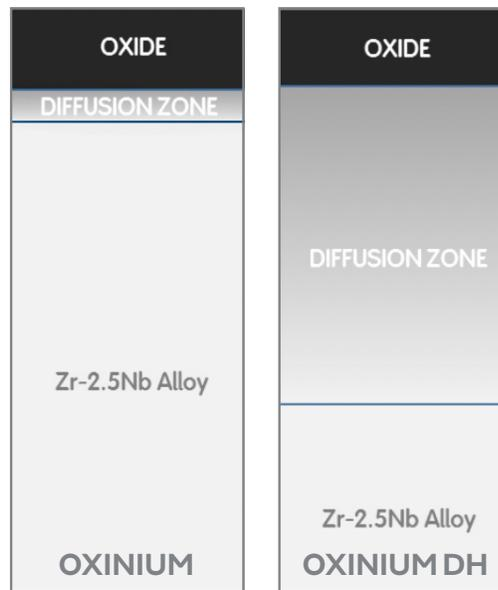
Figure 11: OXINIUM and OXINIUM DH composition
