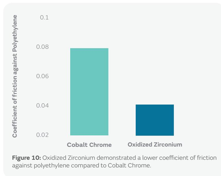
Figure 10: Oxidized Zirconium demonstrated a lower coefficient of friction against polyethylene compared to Cobalt Chrome.
