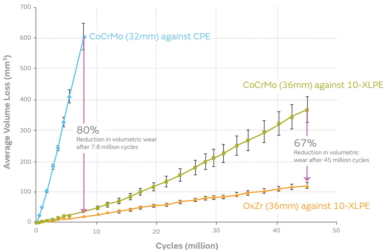
**Figure 8:** Cumulative volumetric wear comparison of CoCr/CPE (blue), CoCrMo/XLPE (green), and OxZr (orange). Error bars graphically represent standard deviation in gravimetric measures of volume loss across all samples.
