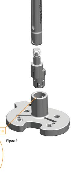
Insert the 3.5mm Hex Screwdriver into the proximal end of the Tibial Trial until the screwdriver is engaged with the hex connection of the Offset Coupler Trial (Figure 10). Unlock the Offset Coupler Trial by turning the hex screwdriver counterclockwise.
